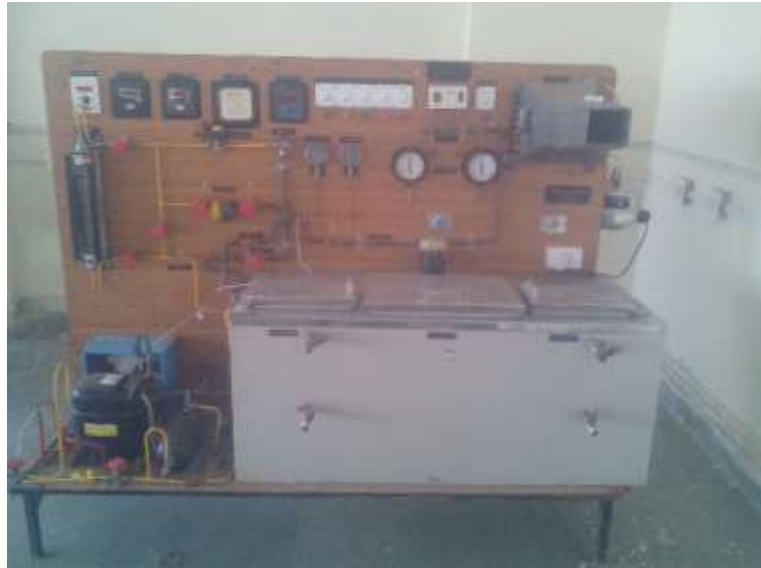
Figure 3 Experimental Refrigeration & Air Conditioning test Rig Unit
